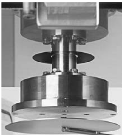
Rotatable, temperature controlled substrate holder with substrate shutter
