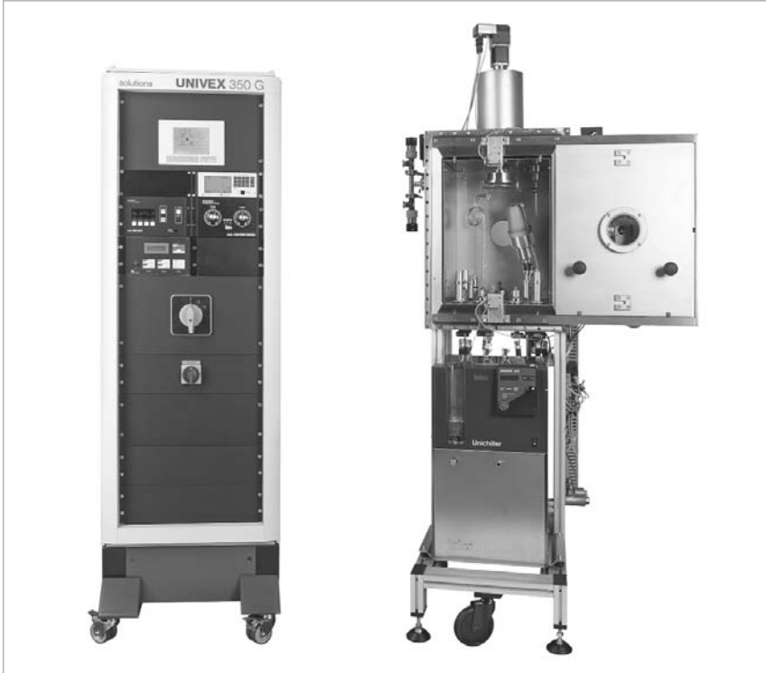
UNIVEX 350 G, consisting of electrical cabinet (left) and coating module (right)
