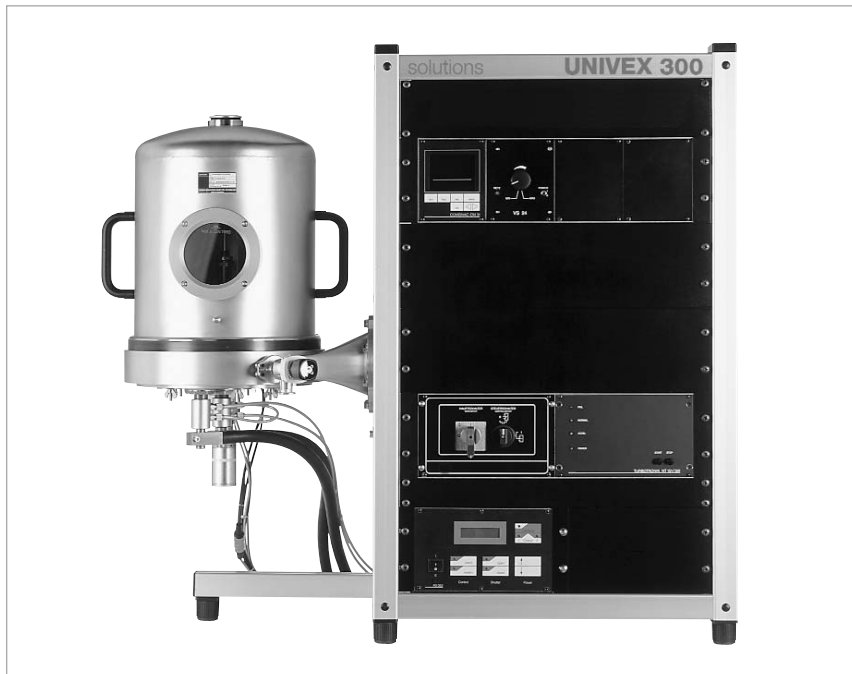
UNIVEX 300, typical arrangement with stainless steel bell jar and process components
