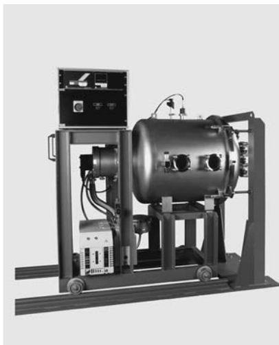
Test system with a 700 mm dia. chamber
